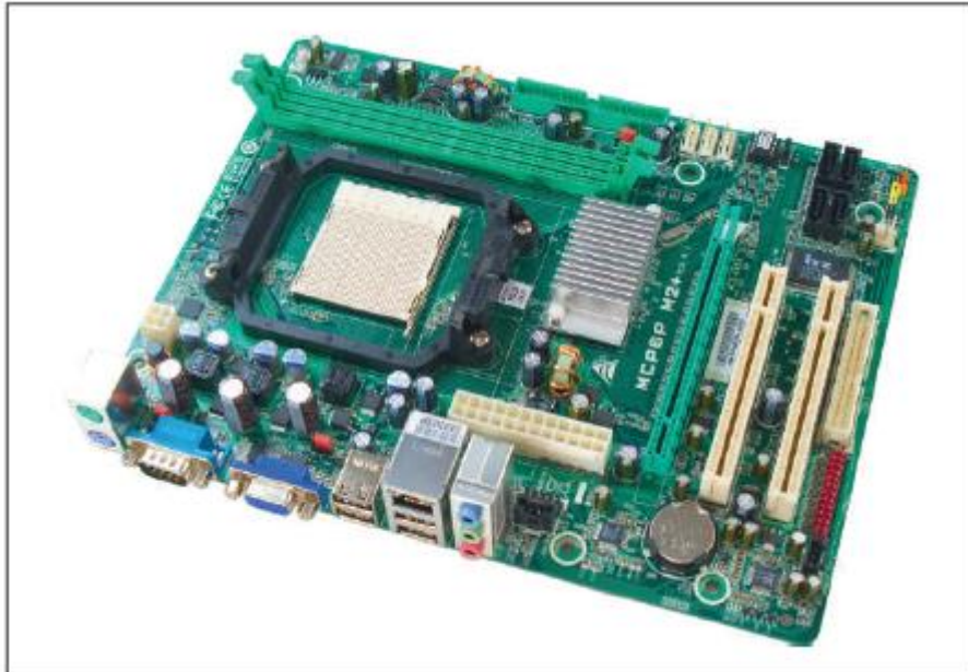
Figure (17) This microATX motherboard by Biostar is designed to support an AMD processor Now let's learn about the drives you might find installed inside a system.
