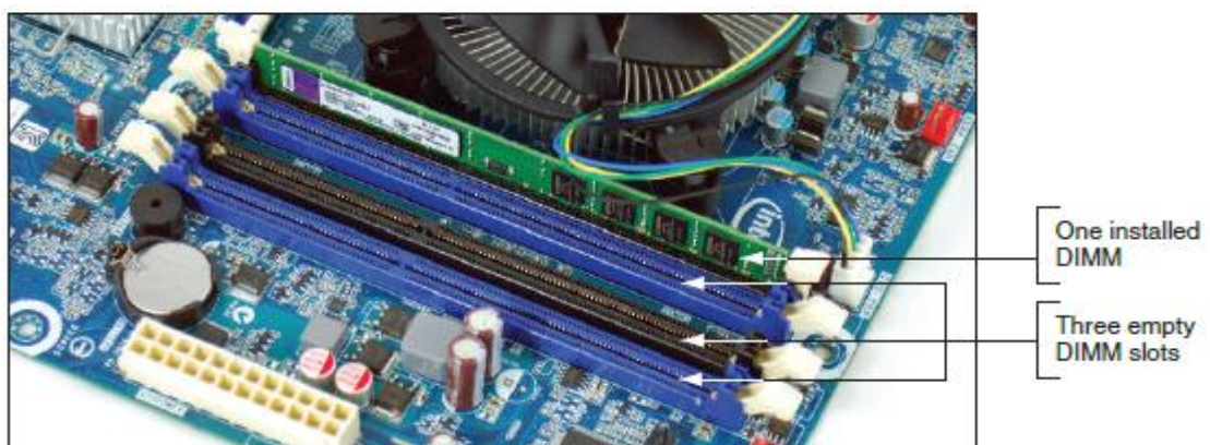
Figure (6) A DIMM holds RAM and is mounted directly on a motherboard
