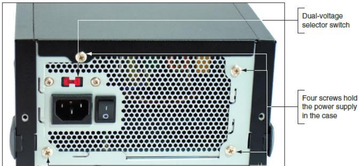
Figure (9) The dual-voltage selector switch sets the input voltage to the power supply
