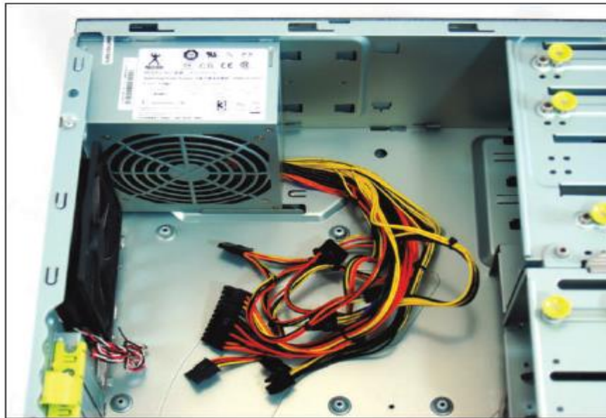
Figure (8) Power supply with attached power cables
