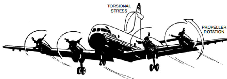
Figure -2.—Engine torque creates torsion stress in aircraft fuselages.
