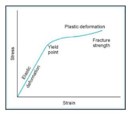
Fig. 2.1: Stress-strain diagram for a solid
