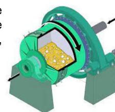
The factor of greatest importance in the operation of the ball mill is the speed of rotation.
