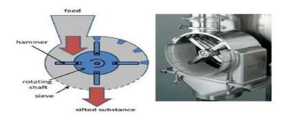
The material is fed at the top or center, thrown out centrifugally, and ground by impact of the hammers or against the plates around the periphery of the casing. The clearance between the housing and the hammers contributes to size reduction.
