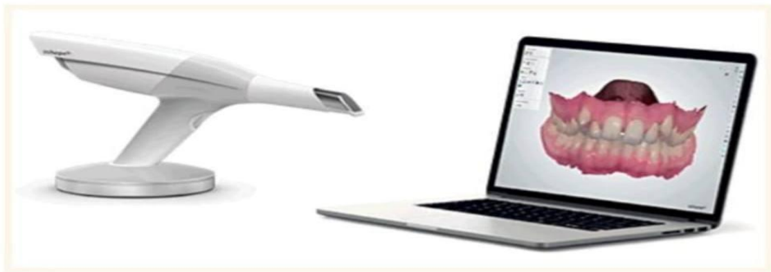
Figure 7 : Iso Device ( Logozzo et al ; 2011 Scans the geometry intra orally and send it into the computer )
